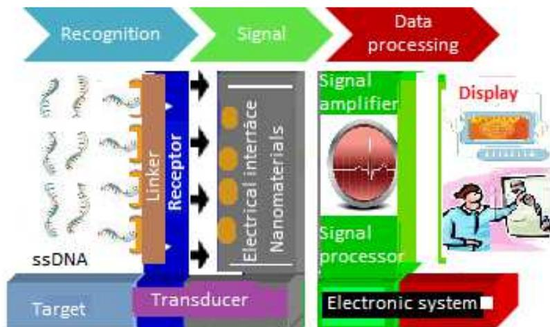
Figure 3: Nanoparticle based halal authentication sensor
